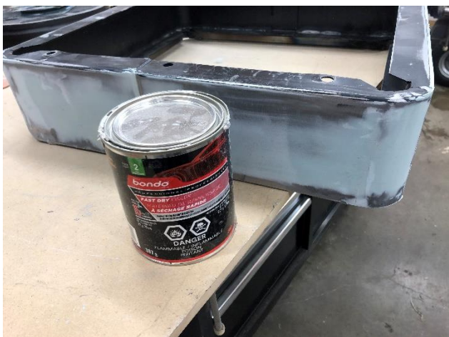
(Grinding the welds smooth, using auto body filler to fill in the imperfections then sanding again made for a satisfactory finish.)
