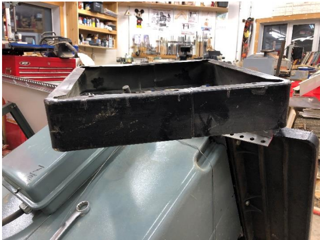
(Fortunately for me, I could tip the table saw on its front and remove the four bolts that held the base on.)
