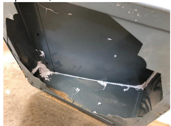
(My Unisaw was not set up efficiently for dust collection. I filled up all the gaps in the sheet metal with silicone so that sawdust does not fall into the base.)
