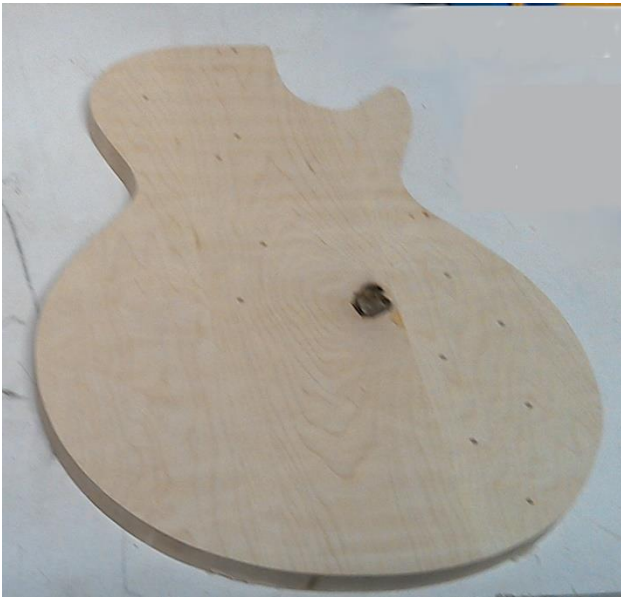
Note pilot holes for the control potentiometers.
