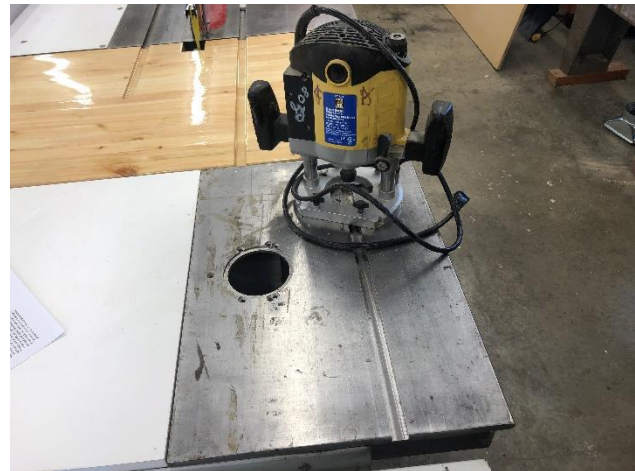
(The steel custom made router table, also constructed 20 years ago installed on the right end of the contractor saw. The Powerfist router that will be installed in it.)
