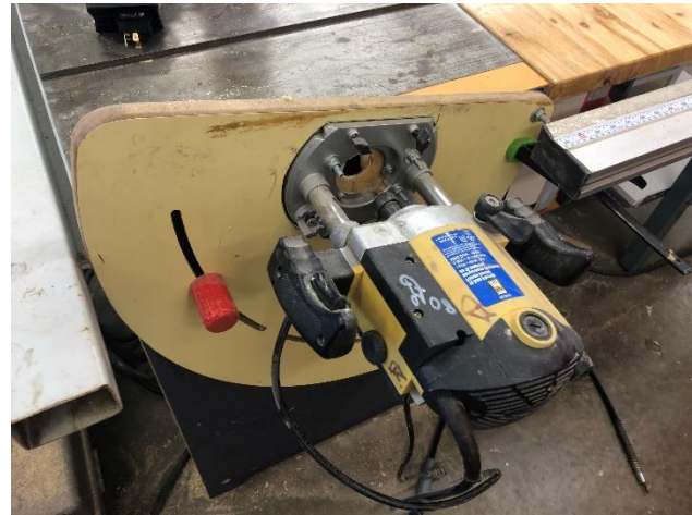
(This horizontal router jig that I built 20 years ago works really well.)
