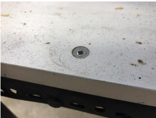
(Quarter inch counter sunk head bolts attach the melamine shelf to the handi-angle sub structure.)
